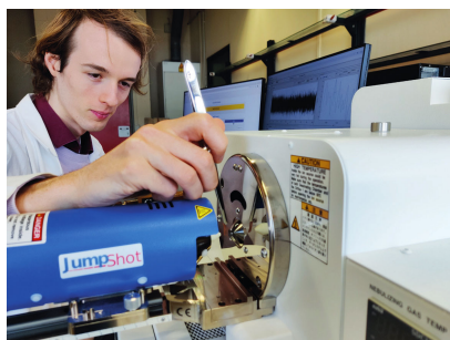
© ENFORCE_RMCA - Chemical analysis of a wood sliver with a mass spectrometer (DART-TOFMS)
